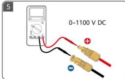
**EN-GB** Recommended connections of DC input terminals
