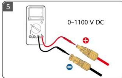
**EN** Recommended connections of DC input terminals
