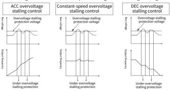
Figure 6-1 Actions taken for protection against overvoltage stalling
