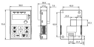
Figure D-4 Keypad external view
