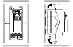
Table 3-1 Installation space dimensions of a single VFD
