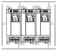
Figure 3-3 Installation space diagram of multiple VFDs
