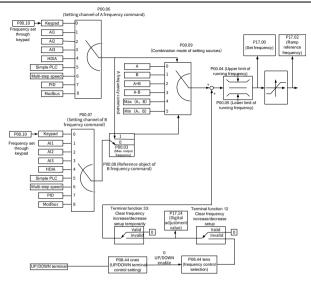
For example, when selecting function 10 or 11 for function code P05.01 or P05.02, S1 or S2 is the Up or Down terminal. When S1 or S2 is closed, the reference frequency increases or decreases quickly. The increase or decrease change rate is determined by P08.45 or P08.46, as shown in the following figure.
