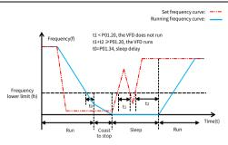
When the set frequency is lower than the frequency lower limit, and the ones place of P01.19 is set to sleep, the VFD stops according to the tens place of P01.19 and sleeps once running at the lower limit for the time specified by P01.34. If the set frequency exceeds the lower limit again and it lasts for the time specified by P01.20, the VFD restores to the running state automatically and increases to the set frequency.
