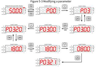
Note: When P00.18 is set to 3, any function code value does not blink, and any function code value cannot be modified.
